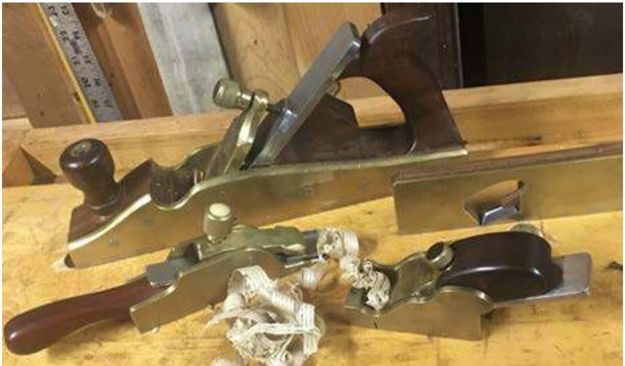
Several Kingshott style planes. The larger plane is a panel plane (jack tuned like a smoother), a half inch rabbet, and a chisel plane made by joining brass sides to a steel sole with through dovetails. The chariot plane is cast bronze with an adjustable toe.
