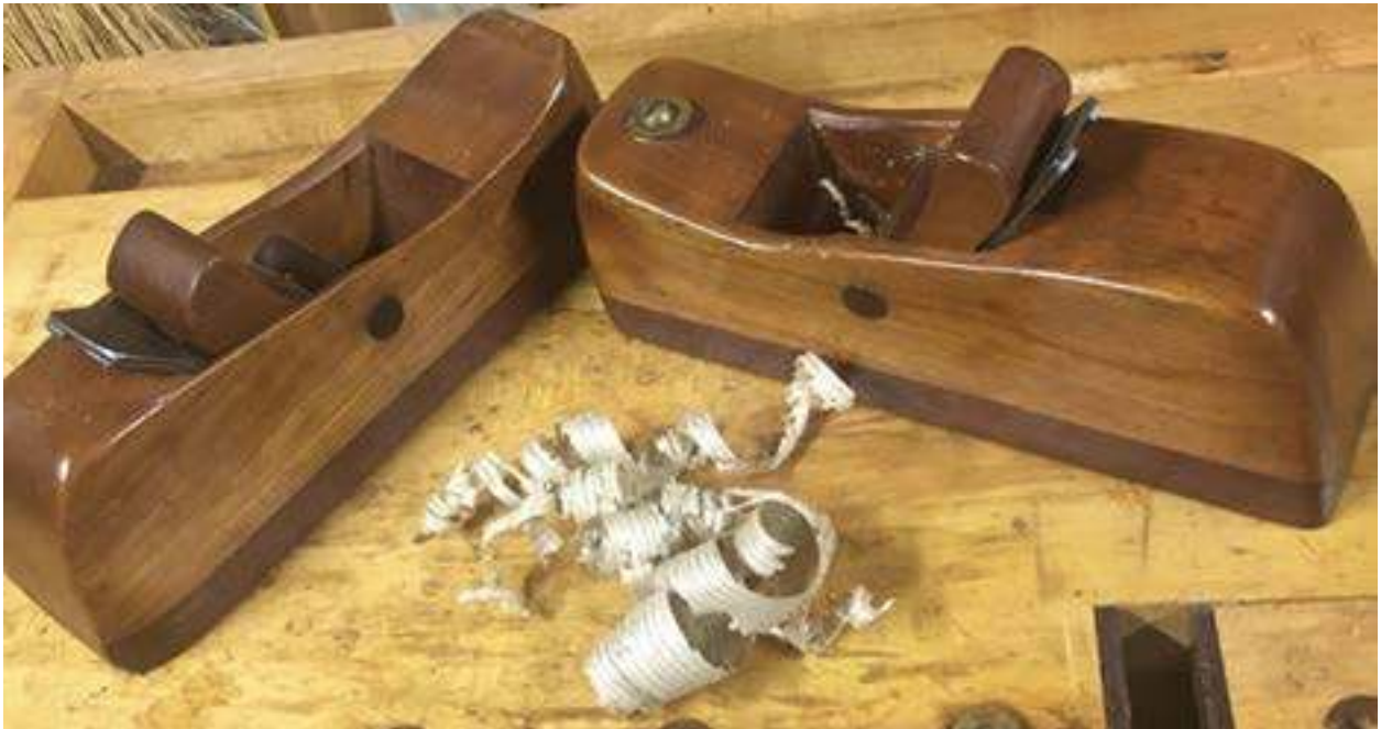
Two Kenrov style planes, one with a 45 degree bed and the other at 55 degrees with an adjustable mouth using a movable toe. Wood is cherry for long term good looks and ease of shaping with a hard bubinga sole for durability.
