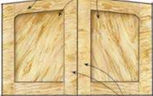
Book-matched inner stiles ensure symmetry and grain flow across gap.
