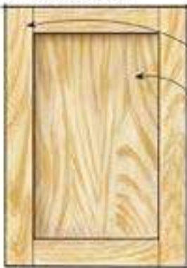
Erratic grain tends to visually distort frame, and may indicate warp-prone wood. Poorly composed edge-joined panel creates messy grain patterns.
