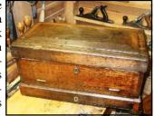
nicely hand made with excellent joinery to house a number of small precision tools while permitting them to be easily retrieved. The molding along the bottom box opens at the front revealing a hidden drawer (of course, the keyhole gave it away).
