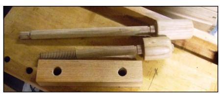
threads (3 inch) may be as little as two to four to the inch though taps and threadboxes are not readily available (certainly not at a reasonable price) over 1.5 inches in diameter. The tap and "V" cutter can be sharpened but last a long time between sharpening when used for personal threading, comparable to the use of a hand saw between sharpening.
