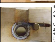
threadboxes the outfeed is threaded wood ... others use a metal (aluminum) threaded insert to reduce wear.
