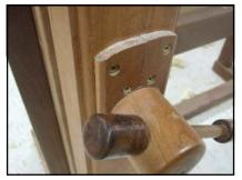
ter groove to about 1/16 to 1/8 in deep. The two pieces are clamped back together and center drilled with a bit the diameter at the bottom of the groove. The two pieces can be placed over the groove and screwed to the moving jaw with two to four wood screws or bolts (see tapping wood for metal bolts elsewhere in this arti-
