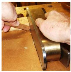
Chamfering the end of the dowel was equally straightforward. I move the plane forward on the shooting board and held the edge of the blade inside the diameter of the dowel. Holding the end of the dowel between the fence and the blade, I angled the dowel at about 45 degrees above the surface of the shooting board and 45 degrees back from the shooting edge. I just rotated the dowel with my fingers to make a nice chamfer to my liking.
