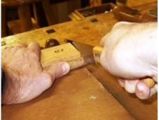
the dowel along the fence and making two or three passes with the miter plane. If you don't have a miter plane most any bench plane or low angle block plane will do as long as the sides are parallel to the sole and the blade is ground flat. The larger the side surface area the better, of course. It would be okay to use a blade with the edges rounded (so as not to dig in when surface planing) as long as the edges
