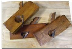
across grain, the shoulder must first be scored with a knife or saw cut or the stock will tear out along the cut. After an initial shoulder is cut the plane will not only track but tearout is less likely as well.
