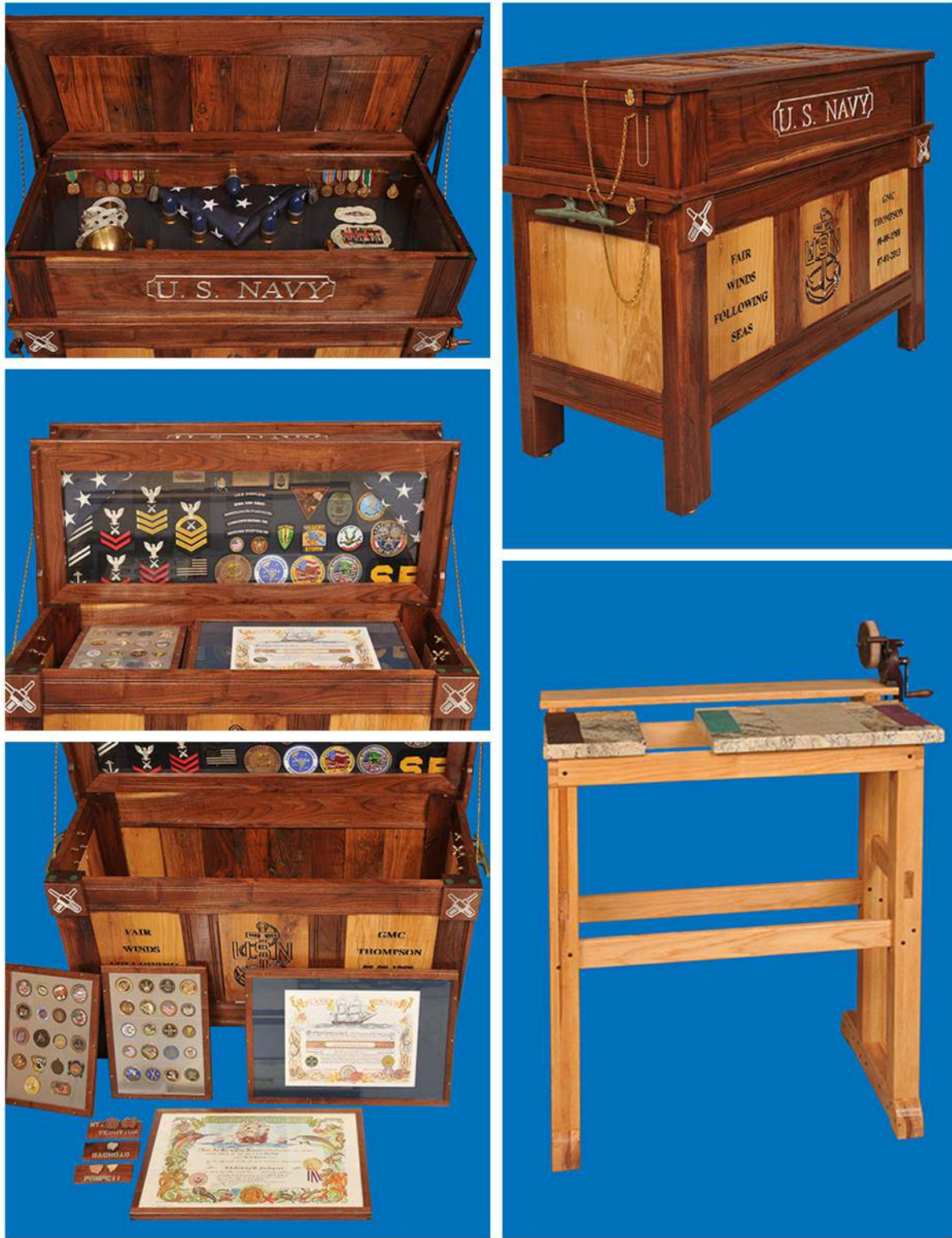
Figure 1: Sharpening Station by Jerry Stanley Made with hickory, granite; Finished with Danish oil, polycrylic; Challenges with dovetails, mortises Shadow Box and Chest by Arnold Baker & Tommy Thompson; Made with walnut, cottonwood, cedar bottom; Finished with Spar varnish oil; Challenges: 150 dowels over 200 hrs; Baker519@att.net
