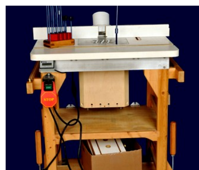
Router Table & Router Lift by John VanGoethem, point of interest used twin screw \frac{3}{4} " - 16 Thread chain drive
