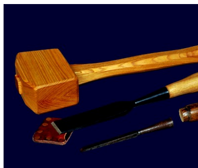
Mallet & Chisels by Bill Rivett made with hickory, finished with linseed oil, challenge was book match head of mallet
