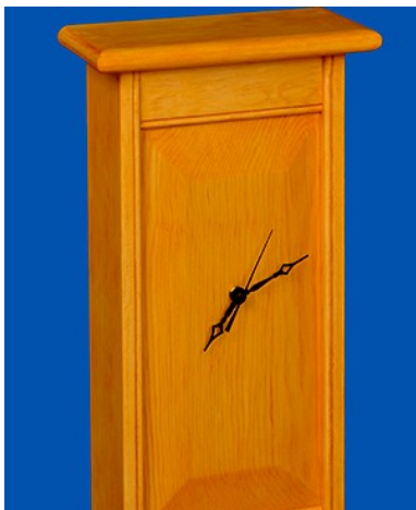
Mantle Clock by Rob Young Made of pine, Finished with shellac & wax Point of interest is it was made with all hand tools except mortise for mechanism
