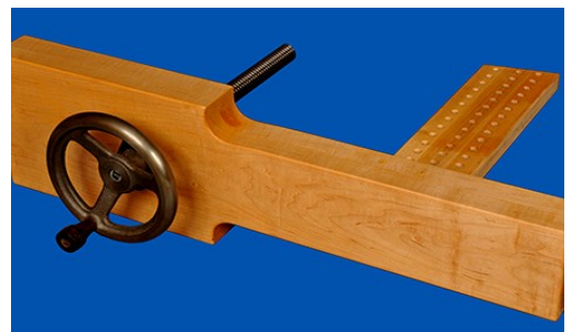
Leg Vise Jaw by Rod Hansen. Made of maple, bench crafted vise. Finished with linseed oil Point of interest from massive 30x84" bench top (split top raubo) Challenges were many
