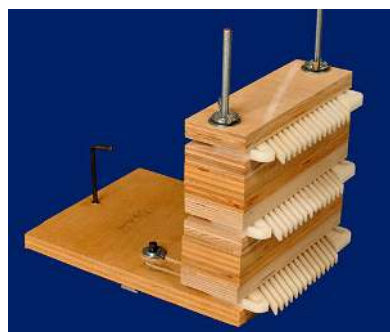
Band Saw Resawing Finger by Russ Amos made with scrap plywood and plastic fingers
