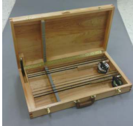
John Tegeler made this Fly Rod & Reel Box with Birch and finish of 3 coats Tung oil. Also has 1 coat wax. Challenges: dove tails, install closer, install rods and reels
