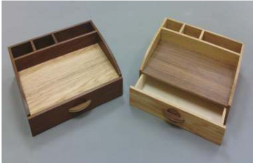
Russ Amos made this Desk/Vanity Organizer with Walnut and Red Oak and Tung oil & Paste Wax finish. Also has hidden compartment. Challenges: Getting all the Rabbits and the Daddos in the right place. 23 pieces made
