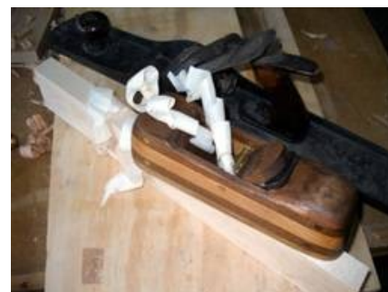
Make a Krenov style wooden body smoothing plane...
