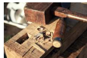
Stop into Rob Young’s Open Shop to experiment with hand cutting the joints with surprising accuracy.
