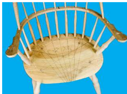
Mark Waugh—sack back chair, red oak, pine and maple—from Windsor Institute class. Note layout marks on seat
