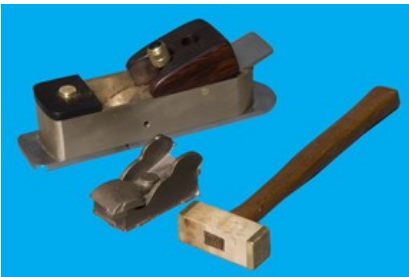
Bill Johnston, infill mitre plane, bronze, brass, carbon steel, cocobola, adjustable mouth
