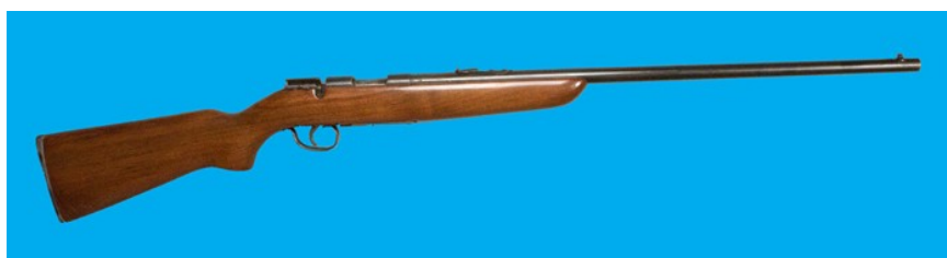
Refinished .22 Rifle Finished Linseed Oil & Varnish Reblued Metal By Arnold Baker
