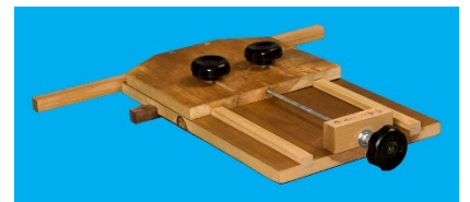
Jerry Jennings—jig for repeatable miters using tablesaw
