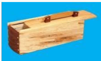
Cliff Schuette wine gift box, ambrosia maple, walnut white oak, Danish oil & wax, challenge getting lid to fit in climate with significant humidity changes
