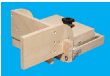
Don Inbody's Tenoning jig made from Baltic birch.
