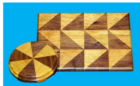
Russ Amos: Trivets made from scrap picture frames. He used scrap from miters on picture frames.
