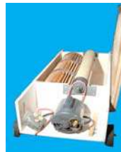
Norm Rechlin's 30" MDF and Birch Ply. Drum sander
