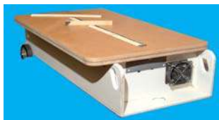
Norm Rechlin's 30" MDF and Birch Ply. Drum sander
