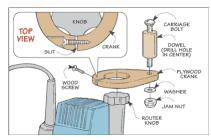
The knob on my plunge router is small and hard to turn. To make it easier to use, I came up with a simple hand crank. The crank is nothing more than a piece of ply-
