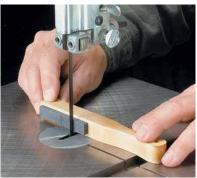
One way to get a smoother curved cut with a band saw blade is to round the back edge with a "tuning" stone (available at <a href="www.Rockler.com">www.Rockler.com</a> or 800-279-4441). With a rounded back, there aren't any sharp cor-
