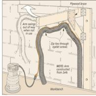
My solution is shown in the drawing at right. I built a simple hinged boom that I attached to the wall of the shop to carry both the power cord and the dust collection hose. When I need the cord and hose, I can
